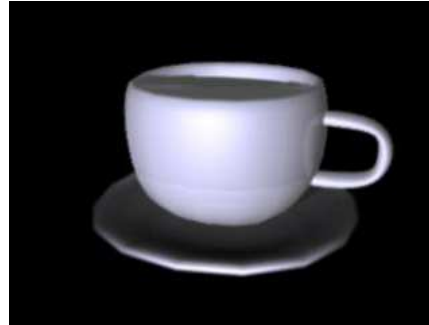
Gouraud (interpolated) shading
