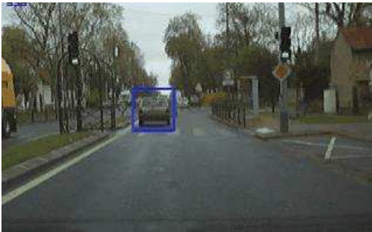
Cars (from behind) : ~ 95% detection with < 1 false alarm / image
