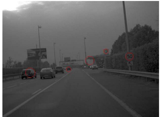
Fig. 3. Example of successful circular sign detection, despite low contrast and luminosity.
