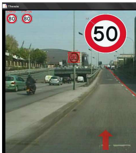
Figure 6. A very interesting case, in which our system correctly determines the 50 limit, even though cartography and vision provide the same wrong answer!
