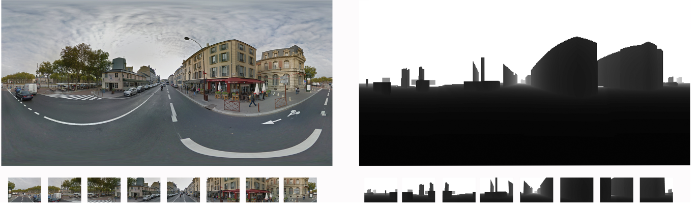
Fig. 1. An example of Street View panorama (top-left) and its associated depth map (top-right) in Versailles, France. The below 8 rectilinear images and depth maps are extracted from the above ones by the back projection. The 8 virtual pinhole cameras, are configured similarly to the vehicle’s camera, including the same focal length and image size. It creates overlapping views.
