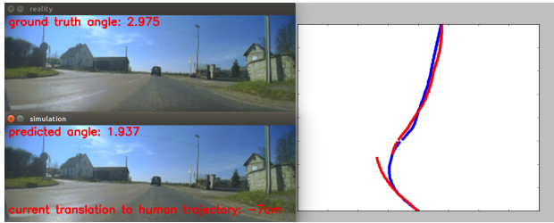
Fig. 5: Screenshot of the simulator, blue trajectory is human, red is the car driven by the network. At current time, the network is translated of 7cm on the right. Here the network failed to take the turn, the red trajectory goes off-road, and a recovery is done.
