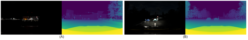
Figure 3: Nighttime Synthetic Drive Dataset examples: (A) depicts HD pattern and (B) high-beam illumination. Ground truth annotations include dense depth maps, semantic segmentation, instance segmentation labels and bounding boxes.
