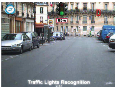
Detection & recognition of Traffic Signs (~95% OK) and Traffic Lights [algos de MINES_ParisTech vers 2011]
